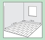
With room lengths of more than 12 m and widths of more than 8 m an intermediate expansion joint should be fitted. Expansion and contraction are linear so the greater the surface the larger the expansion joint needs to be. An expansion joint must be used in typical doorways and room angles. Parquet floors are not suitable for use in damp areas like bathrooms and saunas.
